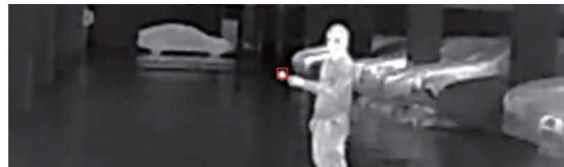
Image by SECT1, detected a fire point from 12m away (match stick, size 8mm×8mm)
